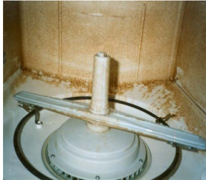
Organic staining inside new dishwasher after three months.
